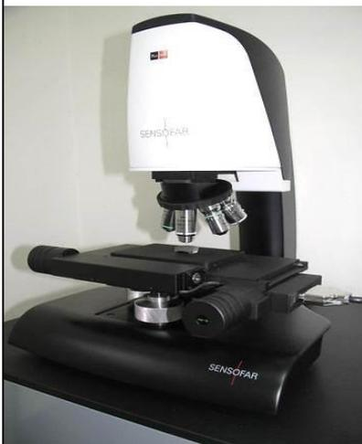
3. **Neox Plu**, confokal mikroskop/optical profilometer (Sensofar, Španielsko) – for the observation and measurement of the parameters of rough surfaces in a magnification 50 – 1500 x with high resolution in Z axis which is suitable for fast measurement of surface roughness (point, line, surface analysis) and cross section profiles (e.g. on wear tracks scratch tests, indentation tests) and coating thickness.
