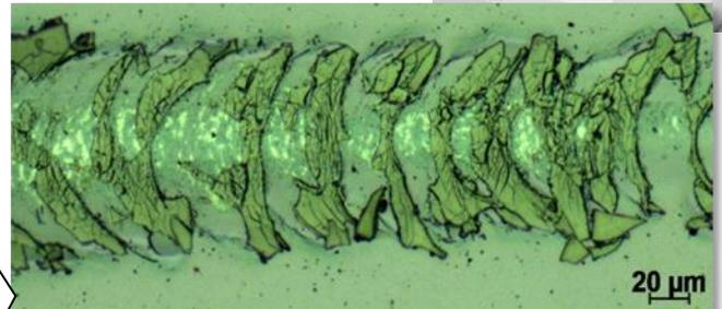
The details of the scratch track after scratch test in a thin coating on a steel substrate using light and confocal microscopy.
