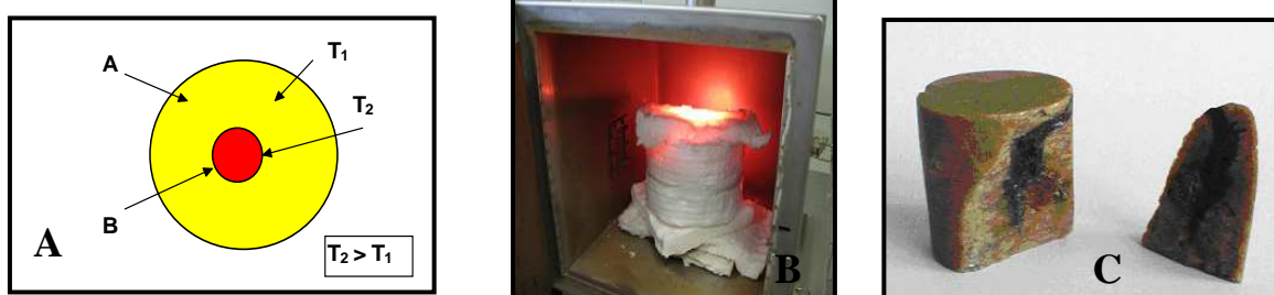
Figure 2: Microwave heating of materials (A), direct heating in a microwave oven (B), and siderite after microwave heating (C).
